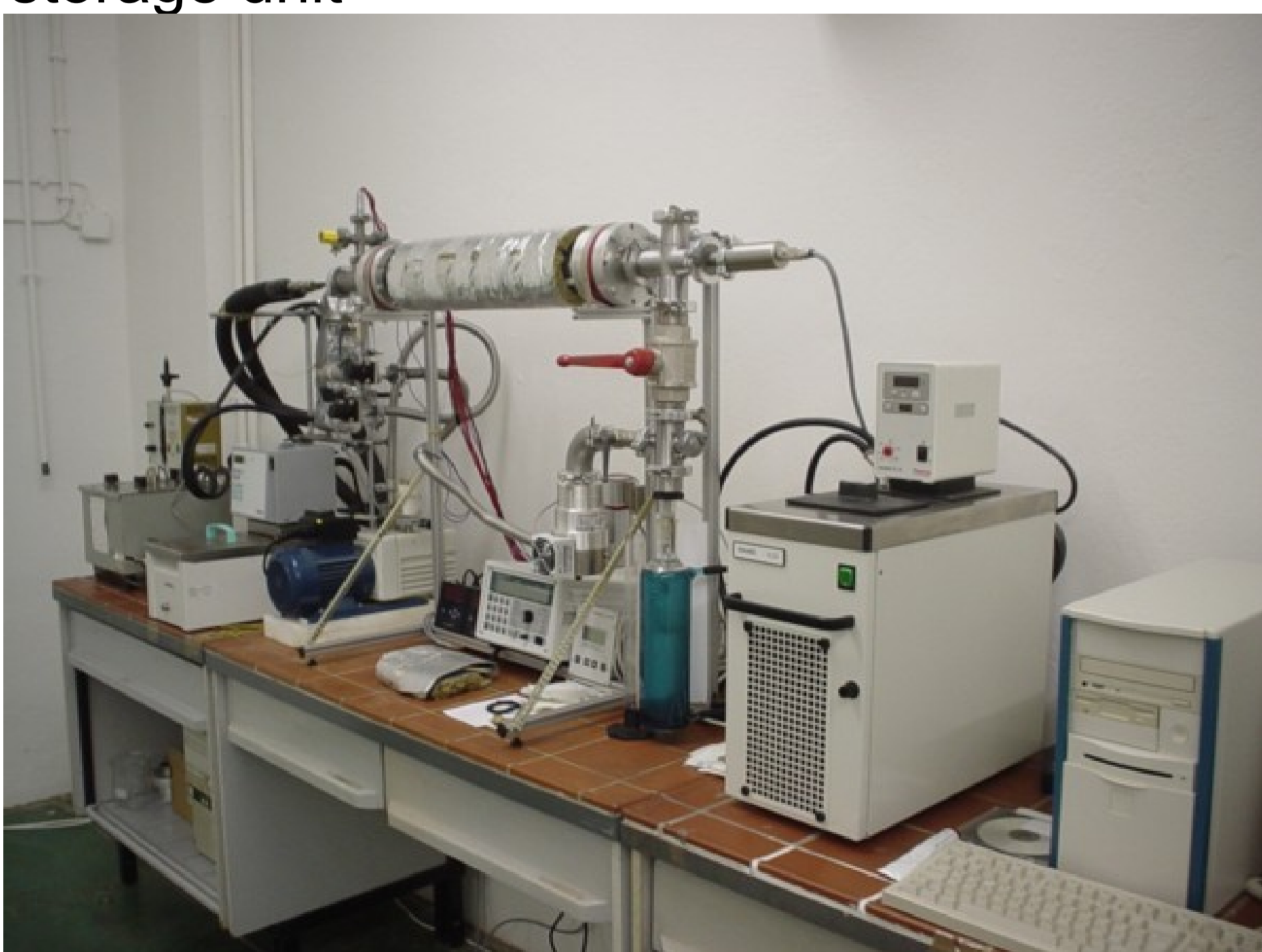
Figure 2: Laboratory scale 1.5 L thermochemical storage unit
